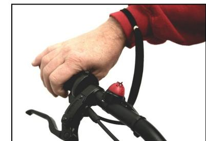
Always ensure the rider is wearing the kill switch around their wrist and that the cord is tightened firmly.
